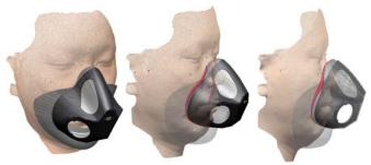
Figure 1. Illustration of a virtual fit analysis of an oxygen mask design on a pilot's face
