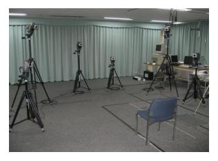
Figure 6. Experimental setup for motion capture
