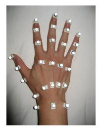
Figure 5. Marker set for hand motion capture
