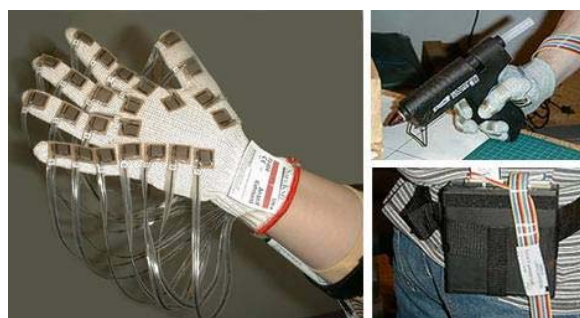
Figure 2. FSA hand force measurement system (NexGen, 2004)
