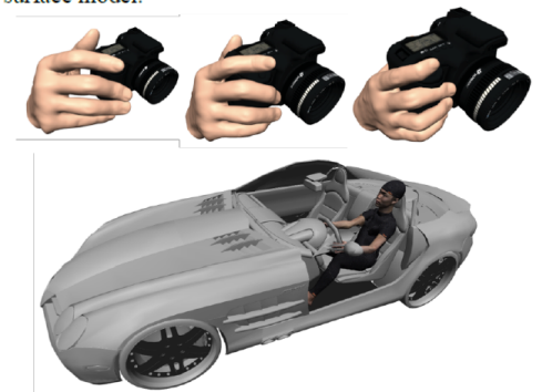
Fig. 8: Results of the posture reconstruction by the simulation using the spring and damper models. Upper left and upper middle figure show the posture reconstruction process. The product models are gradually magnified in the simulation so as to avoid the collision in the early stage of the simulation.
