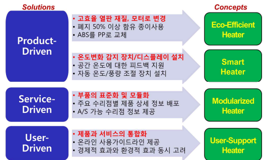
Fig. 2 Eco-design method for electrical small heater
