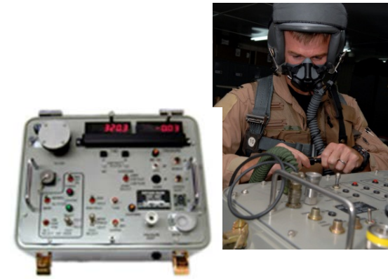
Combined Aircrew Systems Tester (Gentex Corp., USA)
