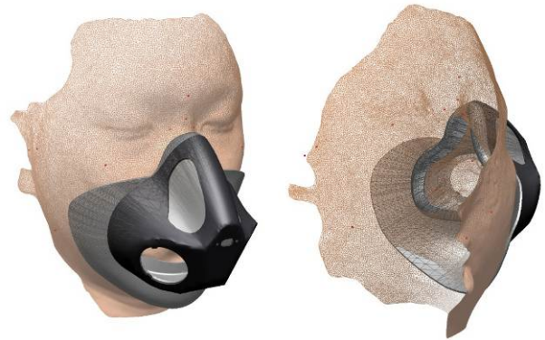
Figure 1. Concept of virtual fit assessment based on 3D facial scan data and oxygen mask CAD
