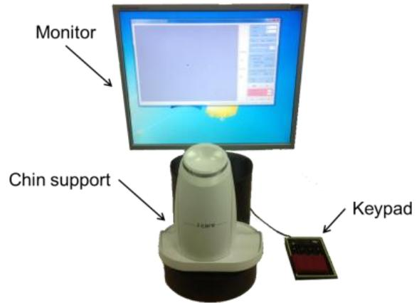
Figure 2. Eye fixation performance testing system - hardware
