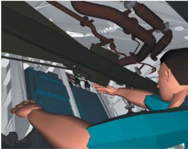
F-22 aircraft maintenance task (removal of an avionics component from the aircraft's weapons bay)
