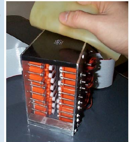
Tactile shape display (Wagner et al.,2002)
