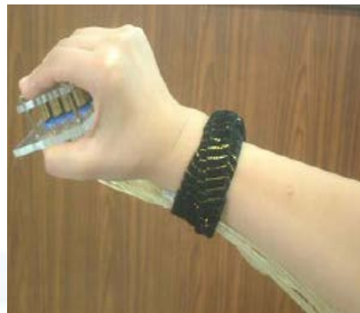
Wearable pneumatic tactile interface (Kim and Ryu, 2005)
