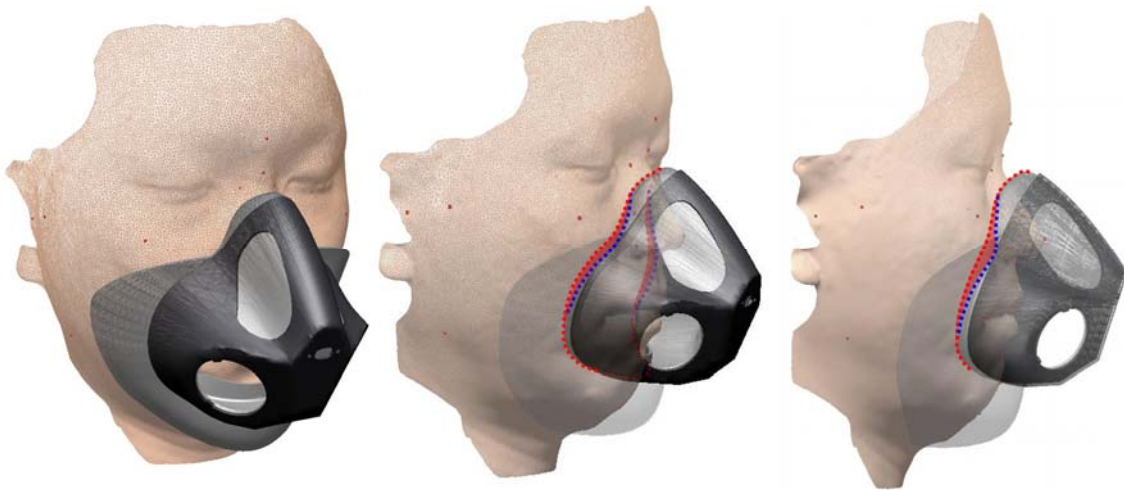
Figure 3.28. Illustration of oxygen mask fit (red area: infiltration of facepiece into face)
