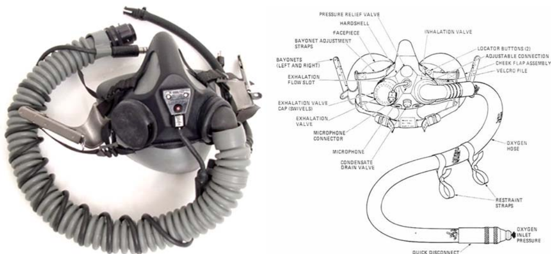
Figure 1.1. Features of MBU-20/P oxygen mask
