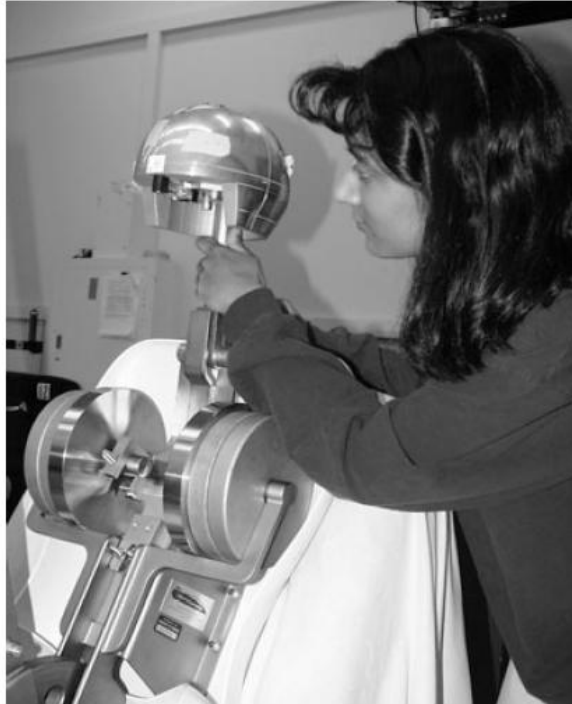
Figure 2.17. Measurement of a head contour using H-point machine (Reed et al., 2001)
