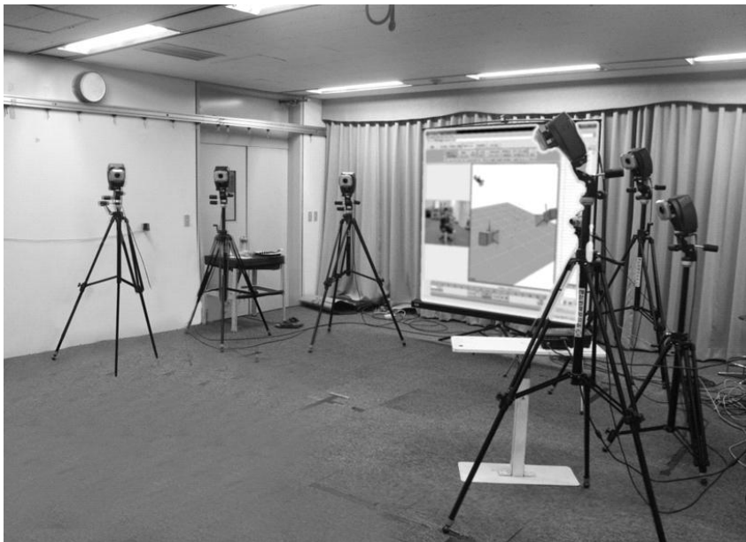
Figure 3.2. Motion capture system to measure a participant's driving posture
