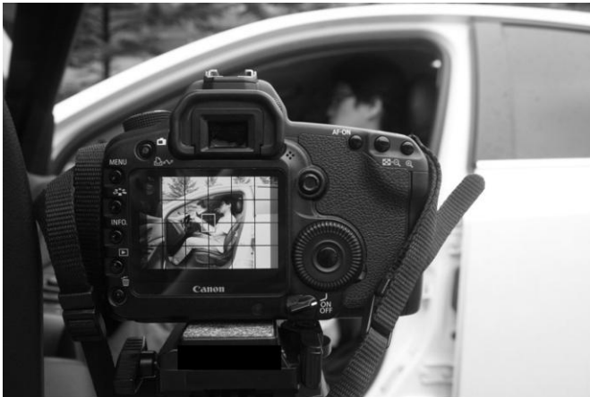
Figure 6.2. DSLR camera set-up to measure a whole-body driving posture
