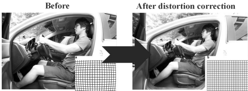
Figure 6.3. Image correction from barrel distortion
