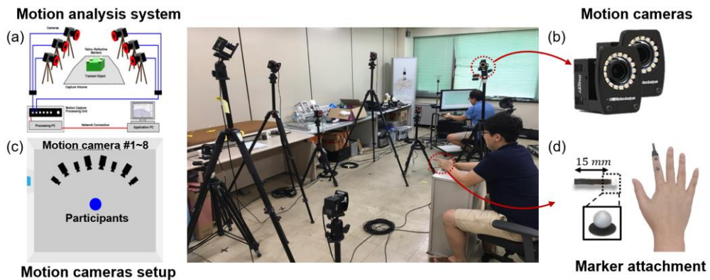
Figure 3.16. Apparatus used in the motion capture experiment: (a) motion analysis system, (b) motion cameras, (c) motion camera setup, and (d) marker attachment
