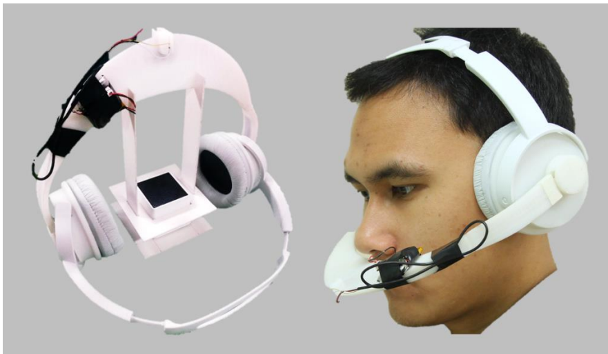
Figure IV.6. The developed nasalance measurement device
